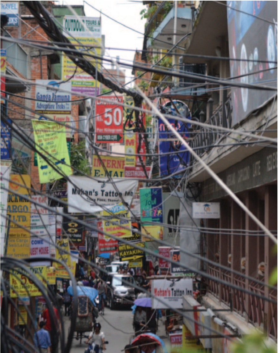
A view down the main street in Thamel from a rooftop cafe. The electricity wires hinder the view and often fall, sometimes catching fire or hitting a passerby. Electricity, produced by hydro power, is rationed with power outages of up to 10 hours a day in the dry season.
